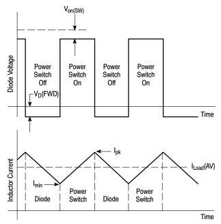
Figure 17. Buck Converter Idealized Waveforms
