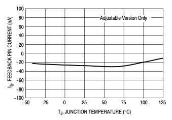
Figure 12. Feedback Pin Current
