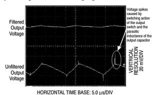
Figure 25. Output Ripple Voltage Waveforms
