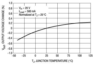
Figure 2. Normalized Output Voltage
