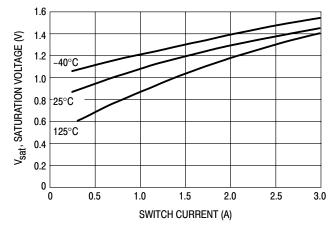
Figure 9. Switch Saturation Voltage
