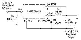
Figure 26. Inverting Buck-Boost Develops -12 V
