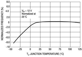
Figure 10. Oscillator Frequency
