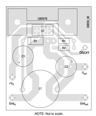
Figure 39. Printed Circuit Board Layout Component Side
