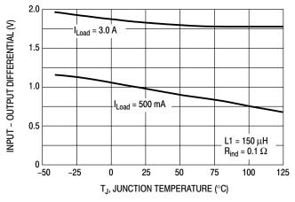
Figure 4. Dropout Voltage
