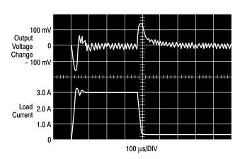
Figure 14. Load Transient Response
