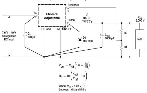
Figure 15. Typical Test Circuit
