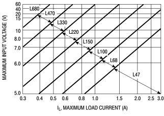
H1000 H680 H470 H330 H220 40 MAXIMUM INPUT VOLTAGE (V) 20 L680 15 12 10 9.0 L100 8.0 **L47** 0.3 0.4 0.6 8.0 1.0 1.2 2.0 2.5 3.0 IL, MAXIMUM LOAD CURRENT (A)
