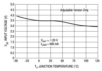
Figure 11. Minimum Operating Voltage
