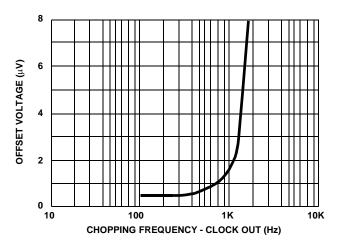
FIGURE 14. INPUT OFFSET VOLTAGE vs CHOPPING FREQUENCY
