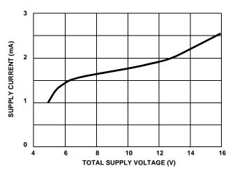
FIGURE 7. SUPPLY CURRENT vs SUPPLY VOLTAGE
