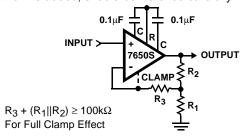
NOTE:  $R_1 || R_2$  indicates the parallel combination of  $R_1$  and  $R_2$ .
