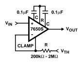
FIGURE 5. LOW OFFSET COMPARATOR
