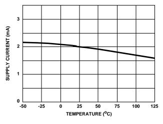
FIGURE 8. SUPPLY CURRENT vs AMBIENT TEMPERATURE
