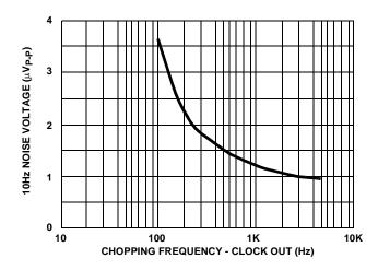
FIGURE 12. 10Hz NOISE VOLTAGE vs CHOPPING FREQUENCY
