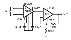
NOTE:  $R_1||R_2$  indicates the parallel combination of  $R_1$  and  $R_2$ . FIGURE 3. INVERTING AMPLIFIER WITH (OPTIONAL) CLAMP
