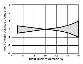
FIGURE 13. INPUT OFFSET VOLTAGE CHANGE vs SUPPLY VOLTAGE
