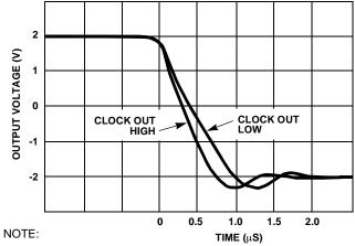
The two different responses correspond to the two phases of the clock.
