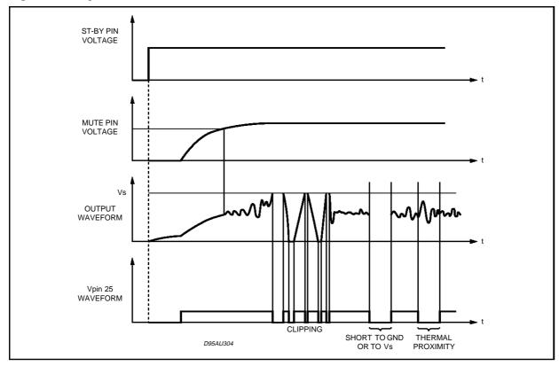
Figure 14: Diagnostics Waveforms.
