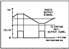
ent feature rather than frequency-dependent. This means that clipping state will be immediately signaled out whenever a fixed power level is reached, regardless of the audio frequency.
