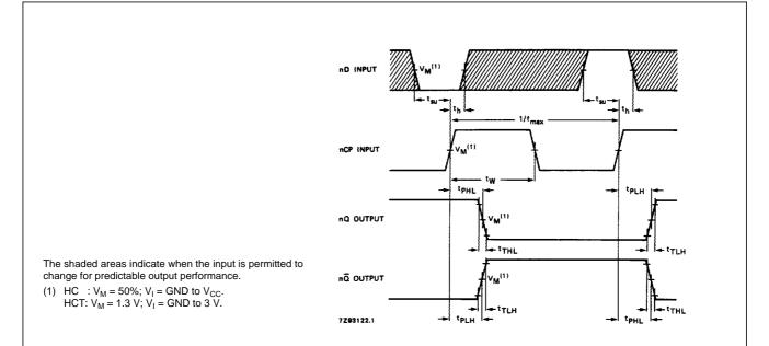
Fig.6 Waveforms showing the clock (nCP) to output (nQ, nQ) propagation delays, the clock pulse width, the nD to nCP set-up, the nCP to nD hold times, the output transition times and the maximum clock pulse frequency.
