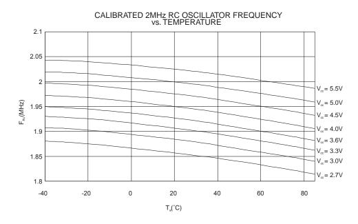
**Figure 151.** RC Oscillator Frequency vs. Operating Voltage (the devices are calibrated to 2 MHz at Vcc = 5V, T=25c)
