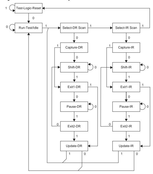
Figure 113. TAP Controller State Diagram
