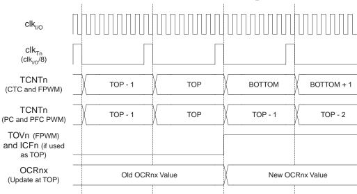
Figure 52. Timer/Counter Timing Diagram, with Prescaler ( $f_{\text{clk\_I/O}}/8$ )
