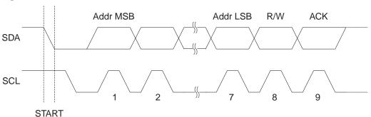
Figure 79. Address Packet Format
