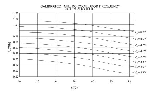
**Figure 149.** RC Oscillator Frequency vs. Operating Voltage (the devices are calibrated to 1 MHz at Vcc = 5V, T=25c)
