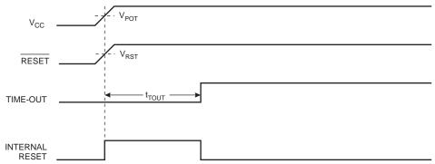
Figure 17. MCU Start-up, RESET Extended Externally
