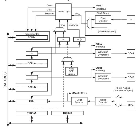
Figure 40. 16-bit Timer/Counter Block Diagram<sup>(1)</sup>
