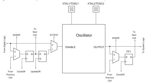
Table 90 summaries the scan registers for the external clock pin XTAL1, Oscillators with XTAL1/XTAL2 connections as well as 32 kHz Timer Oscillator.
