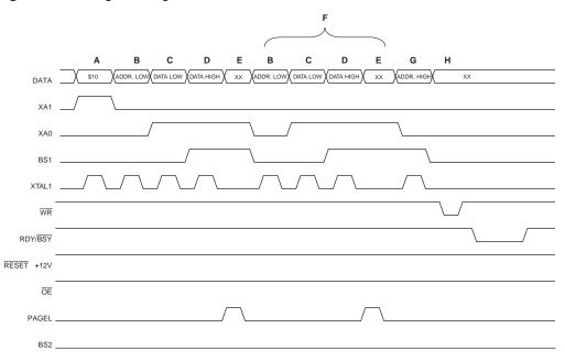
**Figure 129.** Programming the Flash Waveforms<sup>(1)</sup>
