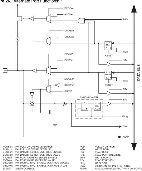
1. WPx, WDx, RRx, RPx, and RDx are common to all pins within the same port. clk<sub>I/O</sub>, Note: SLEEP, and PUD are common to all ports. All other signals are unique for each pin.
