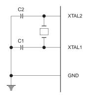
Note: 1. C1, C2 =  $30 \text{ pF} \pm 10 \text{ pF}$  for Crystals =  $40 \text{ pF} \pm 10 \text{ pF}$  for Ceramic Resonators
