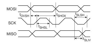
**Table 12.** Serial Programming Characteristics,  $T_A = -40^{\circ}$  C to  $85^{\circ}$  C,  $V_{CC} = 4.0 - 5.5$ V (Unless Otherwise Noted)
