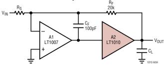
At lower frequencies, the buffer is within the feedback loop so that its offset voltage and gain errors are negligible. At higher frequencies, feedback is through  $C_F$ , so that phase shift from the load capacitance acting against the buffer output resistance does not cause loop instability.
