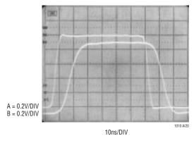
Figure A. Waveforms Using LT1010
