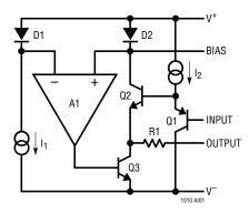
The scheme is not perfect in that the rate of rise of sink current is noticeably less than for source current. This can be mitigated by connecting a resistor between the bias terminal and  $V^+$ , raising quiescent current. A feature of the final design is that the output resistance is largely independent of the follower quiescent current or the output load current. The output will also swing to the negative rail, which is particularly useful with single supply operation.
