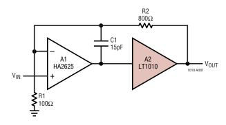
This shows the buffer being used with a wideband amplifier that is not unity-gain stable. In this case, C1 cannot be used to isolate large capacitive loads. Instead, it has an optimum value for a limited range of load capacitances.
