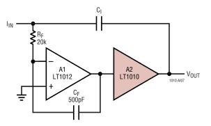
If the integrating capacitor must be driven from the buffer output, the circuit above can be used to provide capacitive load isolation. As before, the stability with large capacitive loads is determined by  $R_{\text{F}}C_{\text{F}}$ .
