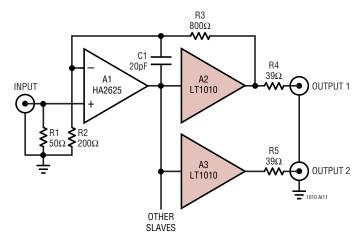
The  $50\Omega$  video line splitter here puts feedback on one buffer with the others slaved. Offset and gain accuracy of slaves depend on their matching with master.
