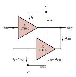
Output load current will be divided based on the output resistance of the individual buffers. Therefore, the available output current will not quite be doubled unless output resistances are matched. As for offset voltage, the 25°C limits should be used for worst-case calculations.
