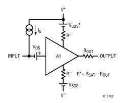
Loaded voltage gain can be determined from the unloaded gain,  $A_V$ , the output resistance,  $R_{OUT}$ , and the load resistance,  $R_I$ , using:
