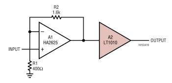
Putting the buffer outside the feedback loop as shown here will give capacitive load isolation, with large output capacitors only reducing bandwidth. Buffer offset, referred to the op amp input, is divided by the gain. If the load resistance is known, gain error is determined by the output resistance tolerance. Distortion is low.
