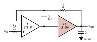
The follower configuration is unique in that capacitive load isolation is obtained without a reduction in small-signal bandwidth, although the output impedance of the buffer comes into play at high frequencies. The precision unity-gain buffer above has a 10MHz bandwidth without capacitive loading, yet it is stable for all load capacitance to over  $0.3\mu F$ , again determined by  $R_F C_F$ .
