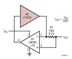
Output resistances of several megohms can be obtained with both circuits. This is impressive considering the  $\pm 150$ mA output capability. High frequency output characteristics will depend on the bandwidth and slew rate of the amplifiers. Both these circuits have an equivalent output capacitance of about 30nF.
