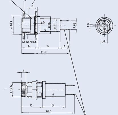
solder/quick-connect terminals 4,8 x 0,5 mm, tin plated, for conductor cross-sections up to 2,5 mm<sup>2</sup> /
